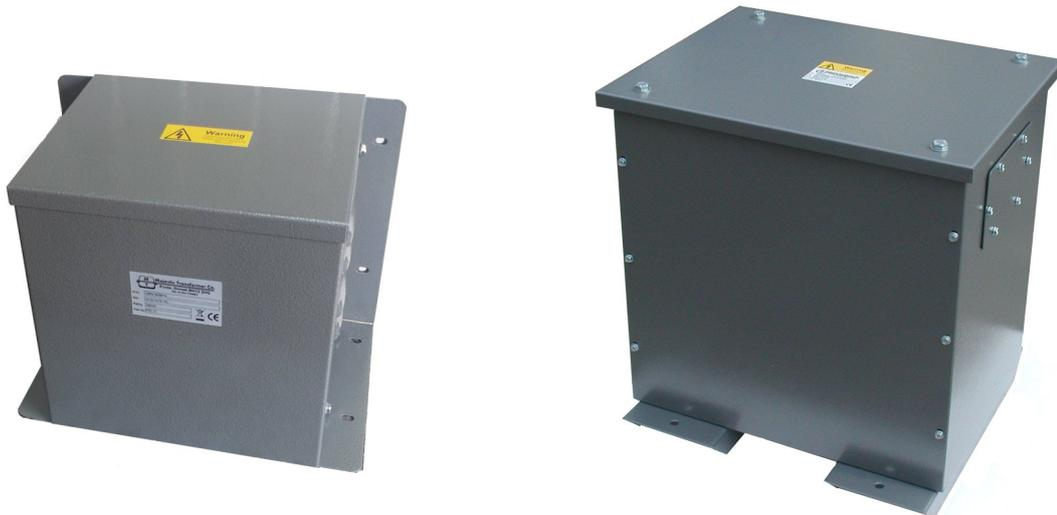
Our transformers in this range are suitably protected by a sheet metal case. They are normally wall mountable up to 6kVA and floor standing above this rating, but a portable style is also available. Many requirements are for low voltage tools or lighting working at 24V or 110V to be fed from mains supplies of 230V or 400V. The above voltages are not exclusive and other inputs and outputs can be accommodated on request.
