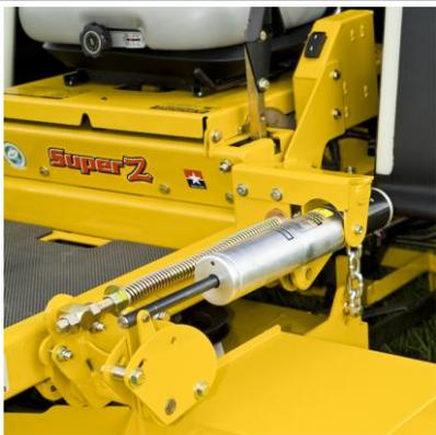
A yellow hydro deck lift mechanism with a hydraulic cylinder and a switch, mounted on a machine's deck. The word 'Super Z' is visible on the side. | <p><b>Hydro Deck Lift</b></p> <p>Raise and lower the deck with the flip of a switch. Fits Hustler Z, Super Z and ATZ.</p>                                                                                                     |
