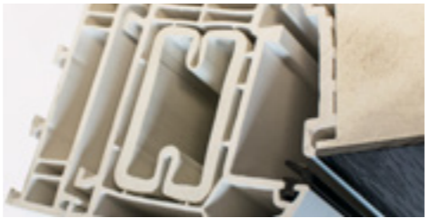
Reinforcement and thickening of door frame The use of reinforcements and local thickening of the door frame provide a stronger fix and improved hardware retention and screw through-pull, locking the sash and frame firmly together.
